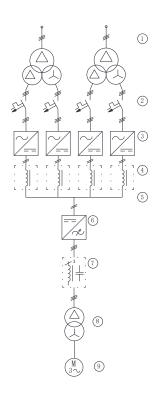
24 Pulse Variable Frequency Drive – The principle of the 24 pulse rectifier has two 12 pulse rectifiers in parallel with two three-winding transformers having a 15° phase shift. The benefit is that practically all low frequency harmonics are eliminated and the harmonic distortion is less than 5%, 24 pulse VFD is IEEE 519 product
